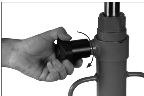
Fig. 5 Rotating the release valve handle clockwise closes the valve.
