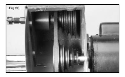
IMPORTANT:- Ensure the wood lathe is disconnected from the power supply before making any adjustments. If you want to increase the speed move the belt outwards. The drive belt can be moved as follows:
