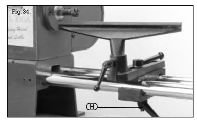
Positioning - (width)- The tool rest can be closer or further away from the workpiece as required. Loosen lever () Fig.35 move to the required position and retighten lever.
