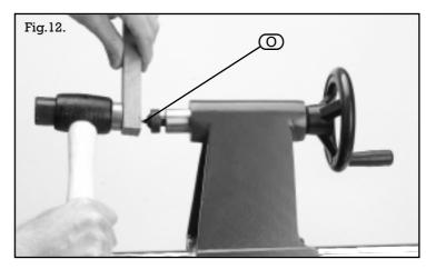
To remove the centre cup from the tailstock barrel insert the ejection pin (supplied), a small wooden dowel or brass rod into the rear of the barrel. Hold the cup with one hand and gently tap the pin with the hammer until it is released. See Fig.13.
