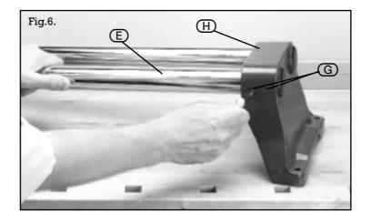
Now slide the bed bars into the headstock and secure by tightening the two hexagon socket head screws ① see Fig.7.
