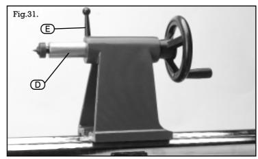
Once in position secure in place by tightening lock knob (E). The tailstock assembly can be moved to any part of the bed bars, loosen locking lever (F) (Fig.32), move to the required position and retighten.
