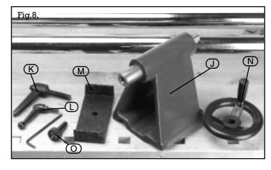
Place the tailstock assembly ① on the bed bars as shown in Fig.9.
