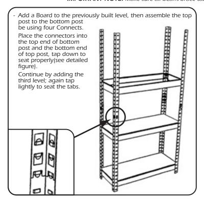
Adding a board shelf to the level previously built, then continue working by adding the final level using two beams and two braces to the unit.
