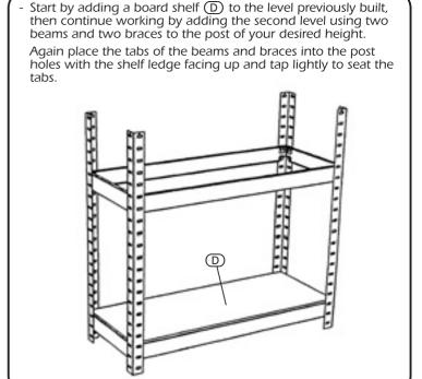
**IMPORTANT NOTE:** Make sure all beam/brace tabs are fully seated into the holes of the post.
