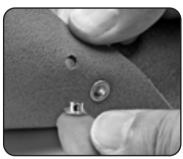
When using the formers, the ready made side of the eyelet should sit in the former with the hole rather than the one with the raised cone. The raised cone forms the other side off the eyelet.
